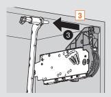
NOTE: Both tabs must be disengaged.
