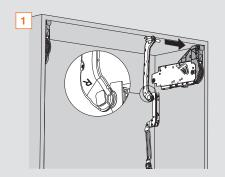
Attach the arm assembly to the lift mechanism as shown in illustrations.
