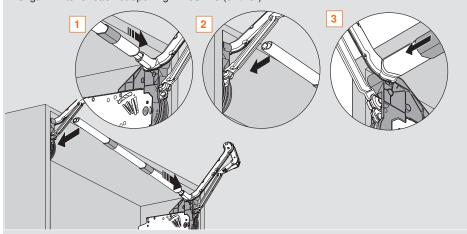
After cutting the rod to size, slide the stabilizer arm cover caps onto the rod. Attach the stabilizer rod to spring loaded arm assembly then slide stabilizer arm cover caps over rod on each end.
