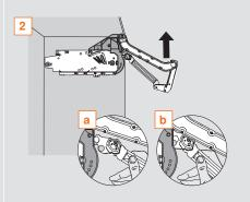
Lift up on the arm assembly to lock into place.
